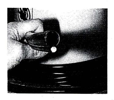
Side view of "ADS" weighted tubing on "Uncoiling Reel". This uncoiling reel is required and can be purchased from "ADS". Notice the "wire keel" is always in the downward position...This is very important to prevent kinking and or twisting of all tubing.
