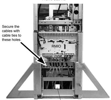
Place for user's motor temperature relay
