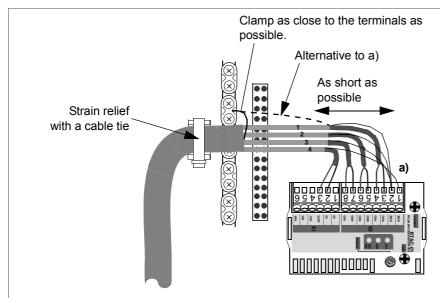
**Note1:** If the encoder is of unisolated type, ground the encoder cable at the drive end only. If the encoder is galvanically isolated from the motor shaft and the stator frame, ground the encoder cable shield at the drive and the encoder end.
