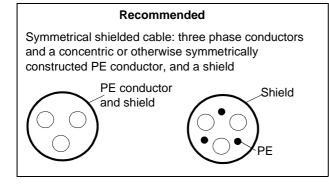
A separate PE conductor is required if the conductivity of the cable shield is < 50 % of the conductivity of the phase conductor.
