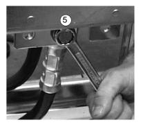
Frame sizes R7 and R8: M12 (1/2 in.) bolt Tightening torque: 50...75 Nm (37...55 lbf ft)
