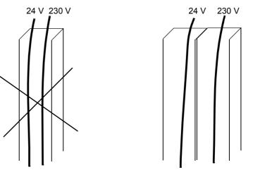
Not allowed unless the 24 V cable is insulated for 230 V or insulated with an insulation sleeving for 230 V.
