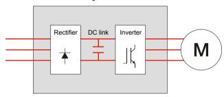
The single drives are complete AC drives that can be installed without any additional cabinet or enclosure. The single drives are available as wall-mounted, free-standing and cabinet-built constructions. The standard protection class of the single drives is UL Type 1 and higher protection classes are available as an option.
