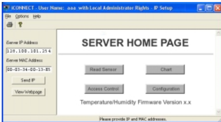
Figure 4.3 Accessing the iServer for Configuration
