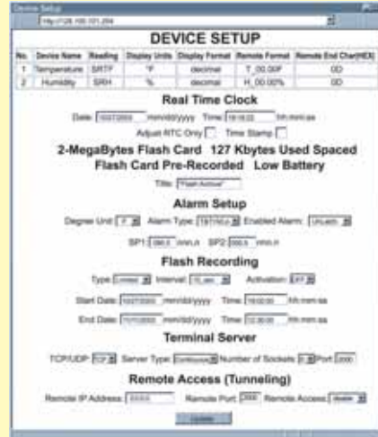
iTHX-M device configuration through embedded Web server.
