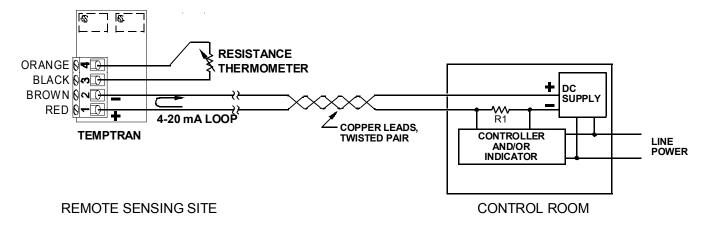
**Installation** of TT210, TT211, TT710, and TT711 Temptrans<sup>TM</sup> in Class I, Division 1 or 2, Groups A, B, C, and D hazardous locations.
