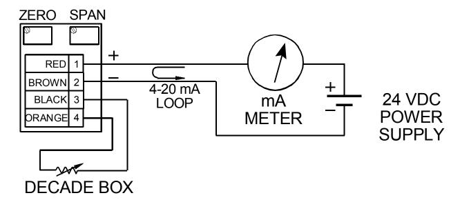
NOTE: Zero and Span resistance values are printed on the transmitter's label.
