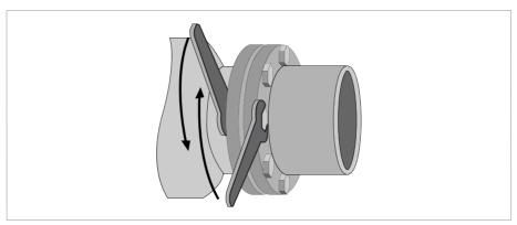
Figure 3-14: Tightening of bolts
