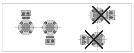
Figure 3-3: Mounting position
