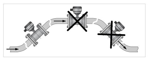
Figure 3-9: Installation in bending pipes
