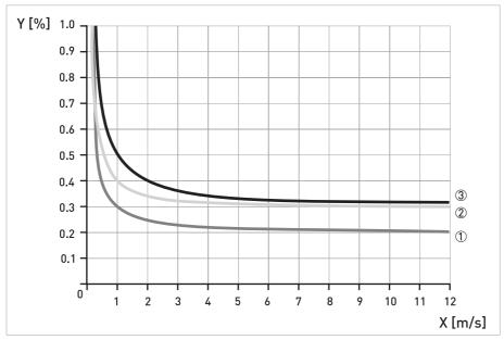
Figure 6-3: Flow velocity vs. accuracy
