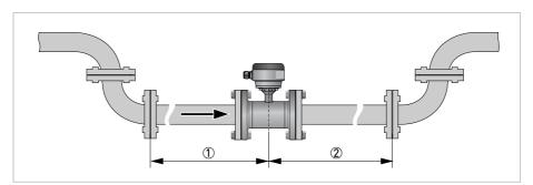
Figure 3-2: Recommended inlet and outlet
