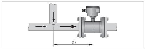
Figure 3-5: Distance behind a T-section
