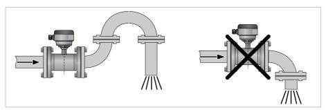
Figure 3-10: Installation in front of an open discharge
