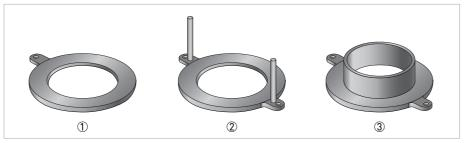
Figure 4-2: Different types of grounding rings
