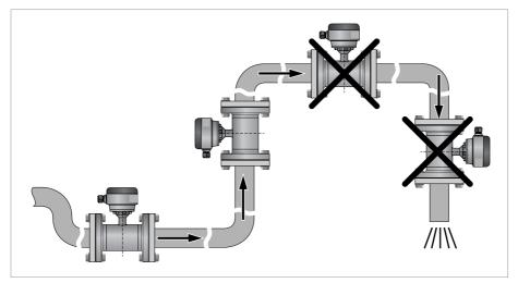
Figure 3-8: Installation in bending pipes
