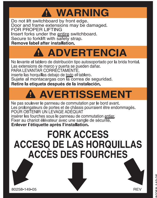
Figure 2: Warning Label, Rainproof Switchboards
